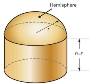
b. Compare the solidification time of the riser you designed to that of a riser shaped like a simple cylinder. Assume that the volume of each riser is the same ( $V = V_s$ , where  $V$  is the volume of a cylindrical riser with height equal to its radius and  $V_s$  the volume your optimized riser).
